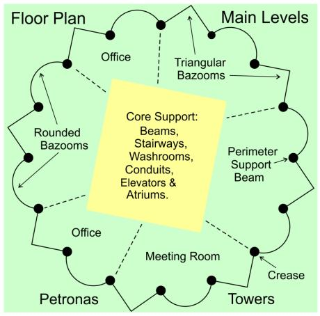
The tower's perimeter maintains the same shape from ground to pinnacle, though the bazooms shrink as the building narrows in the upper stories. The design is an Islamic motif where two squares are superimposed 45° from each other, making an eight-pointed star with eight-square corners. Between each pair of corners lies a rounded bazoom, so the perimeter mimics a corrugated circle with sixteen outcrops.
